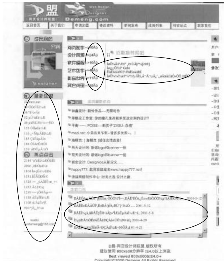
Fig. 1: A page that contains frames with charset tag undefined. The contents in the ovals are not displayed correctly. www.demeng.com
